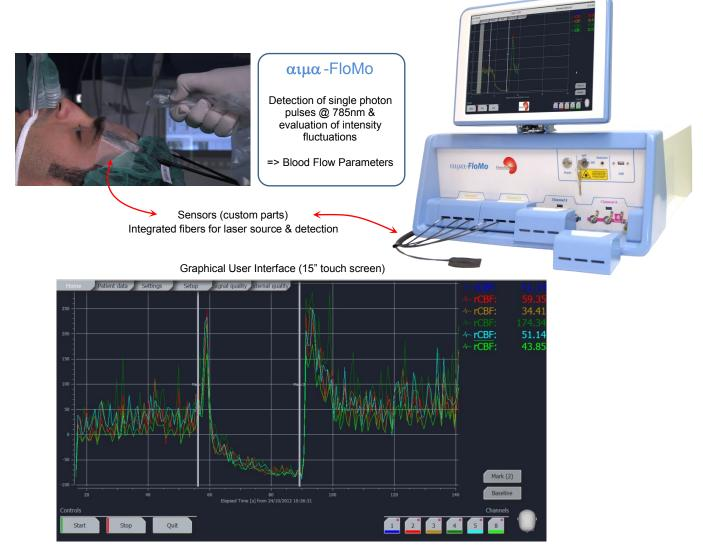
The  $\alpha_{i\mu\alpha}$ -FloMo is meant to be used with an NIRS/DOS system and can readily be integrated with most commercial and custom systems. Together with NIRS/DOS, the blood oxygenation and blood volume (Hb, Hb,THb and StO<sub>2</sub>) can be measured as well as the blood flow which allows the derivation of other relative parameters such as the oxygen extraction fraction (OEF) and cerebral metabolic rate of oxygen extraction (CMRO<sub>2</sub>).
